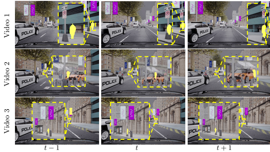
Fig. 4: Qualitative results of the proposed S-AModal method for three sequences \mathbf{x}_{t-1}^{t+1} with overlaid colored amodal predictions \mathbf{a}_{t-1}^{t+1} on AmodalSynthDrive \mathcal{D}_{\text{ASD}}^{\text{val}} .
