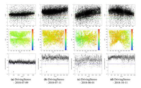
Fig. 6: Visualization of the vertical disparities  $d_y$  and their mean values for training sequences from *DrivingStereo*. The diagrams show different error shapes. Compared to *DSEC* (Figs. 5c and 5d), *DrivingStereo* shows similar error magnitude.
